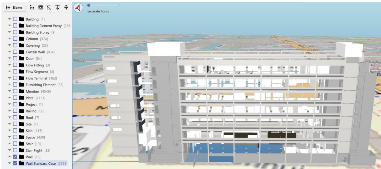
Figure 5: Building with only the elements ‘Wall’ and ‘Wall Standard Case’ enabled
